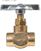
The V1 Series Needle Valve has a 37° medium tipped stem to offer rapid shut off, full flow and a semi-metering function. It is constructed from a forged brass body, brass stem, thrust washer cap, and an O-ring seal.
